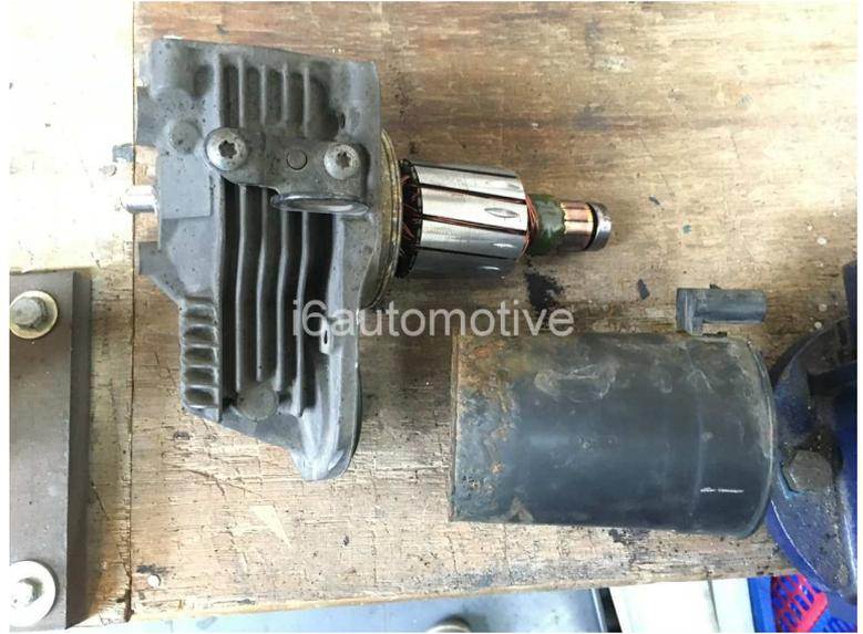
Remove the allen bolt so that you have access to the other side of the electrical unit so that it can be pressed out.
