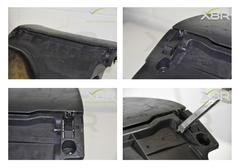
Step 2: Fixing the broken hinges Glue the hinges back onto the glovebox lid, this will help locate the brackets in the next step.
