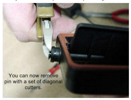
Here is the steel pin removed. It's pressed in pretty tightly on a new unit. This is what has ruined a few engines after it fell out and went through the intake runner and into the combustion chamber.
