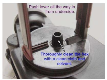
Push the lever all the way in as far as it will go. It should look like this and will probably have grease on the tapered hex section from pushing it through the bearing. While keeping the bell crank pushed in with your finger from the opposite side, completely clean the protruding hex taper with a clean cloth and solvent. Use brake cleaner, acetone, or similar solvent.
