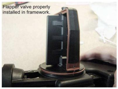
View of the new flapper valve properly in place. Center the flapper to the opening in the top support bearing.
