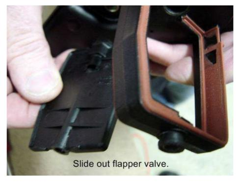
Now that you have the DISA disassembled you will want to clean the DISA housing. I recommend using a full strength industrial cleaner like Simple Green or Purple Power from Auto Zone. I would avoid brake cleaner or solvents as they can make the plastic brittle. Note the little hole pointed to in the picture, this is the vacuum port that actuates the DISA. Plug this with a tooth pick or something to
