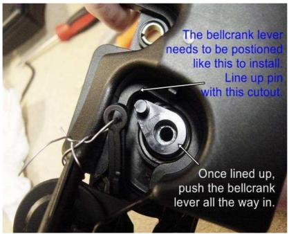
Next, make sure that the bell crank lever is still aligned like this and that the flapper valve is perpendicular to the support framework, then push the lever into place as far as it will go.
