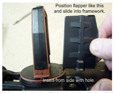
Now you can slide the new valve into place. This is the only orientation that will allow the valve to slide in due to it's shape. It goes in from the side with the vacuum hole with the valve positioned as shown. It's designed to be a precision fit so it needs to be straight in order to slide in.
