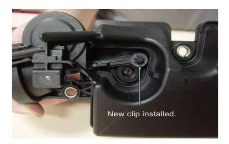
You can now reinstall the plastic cover and you're finished with the valve portion of the install.
