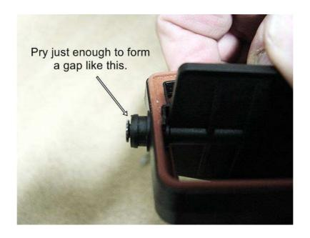
Now you can remove the pin with a small pair of diagonal cutters.
