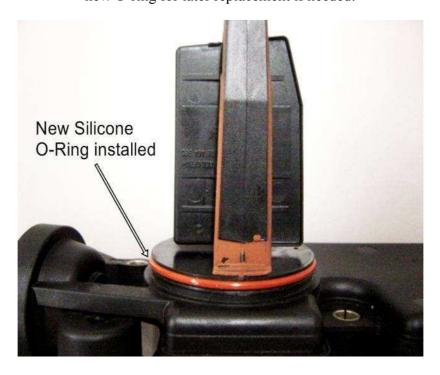
Once the groove is cleaned you can install the new O-ring. Squeeze some of the supplied grease onto your fingers, then work the grease onto the surface of the O-ring before installation. This not only
