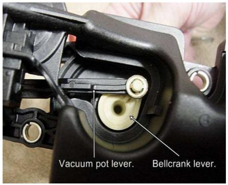
This is what's under the cover. The creme colored piece is the bell crank lever which rotates the flapper valve. This is the piece that typically wears out and causes most of the problems. The black piece is the lever that connects the vacuum pot diaphragm to the bell crank lever.
