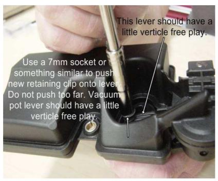
You can now put the vacuum pot actuator lever back over the pin of the new bell crank lever and push the new retaining clip on. Use a socket or other similar tool to push the clip onto the pin. DO NOT push the clip on as far as it will go. Go slowly, you want the vacuum lever to have a little bit of vertical free play. If you push it on too far, pull it back a little with a pair of needle nose pliers while twisting the clip.
