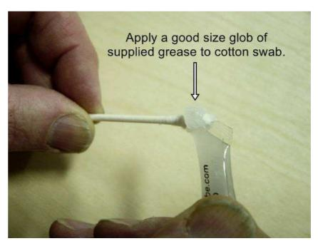
Apply the grease to the inner lip of the bell crank seal as shown. Spread it around inside the lip of the seal.
