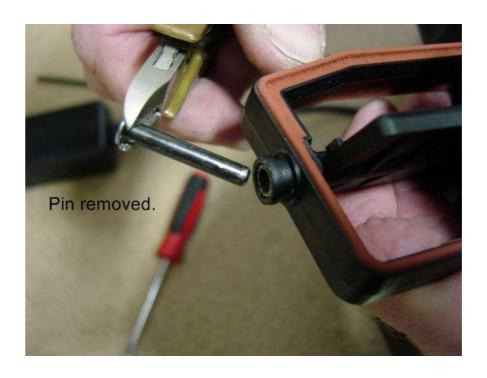
Once the steel pin has been removed, the flapper valve can be slid out of the DISA housing frame work.
