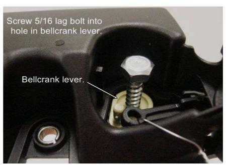
Next you will be removing the bell crank lever from the housing. Start by screwing the supplied 5/16 lag bolt into the hole in the bell crank lever as shown. If you don't have a 1/2 inch or 13mm wrench or socket, this can easily be accomplished with a pair of pliers. Note the installed height shown and refer to the next picture as well. You will not be screwing the bolt all the way in. Just a couple of full turns is sufficient.
