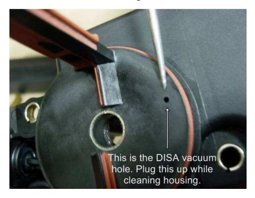
Now that it's all cleaned up, give it one more visual inspection for sizes of damage. Cracked or broken plastic is bad, worn or small missing sections of the orange rubber seal is OK.
