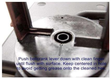
Next, with a clean finger, push the bell crank back down until it's flush with the surface as shown. Be careful, the goal is to keep the tapered hex portion centered in the hole so that you don't get any grease on the taper again. The seal will hold it centered in place once it's pushed down.
