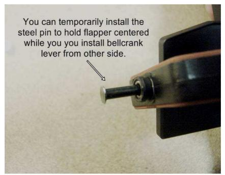
Next you will be pushing the bell crank lever into place. If you want you can temporarily replace the steel pin and hold it in with your finger while you push the bell crank lever into place. This is not necessary, but it helps to keep that end centered while working on the other.
