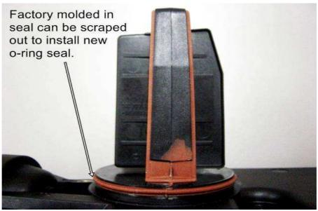
Now that the new valve assembly is installed, all that is left is to replace the main housing seal. The M54 has the main seal molded into the framework which is why BMW doesn't offer a replacement Oring. The old seal needs to be scraped out.
