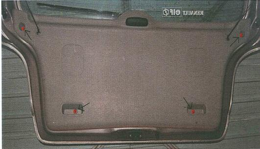
Open the boot and, using the T-20 Torx screwdriver unscrew the four screws, which hold the interior boot trim in place (some models have an additional two screws near the wiper motor). Unhook the parcel shelf bungees from the trim. To remove the trim, pull firmly all around the edges, you will hear a snapping sound, this is just the clips that hold it in place.
