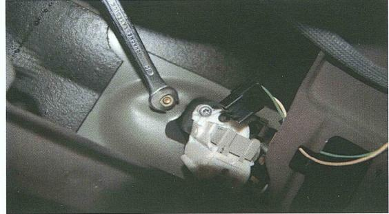
Disconnect the plug from the lock motor and using the 10mm spanner, undo the two fastening nuts which hold the lock assembly to the tailgate panel.
