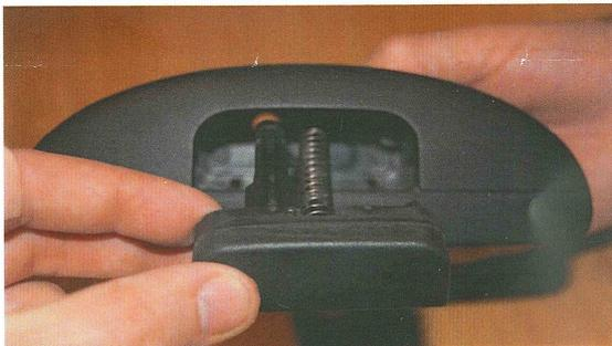
Line up spring and push the long piece through the hole so it sticks out the back
