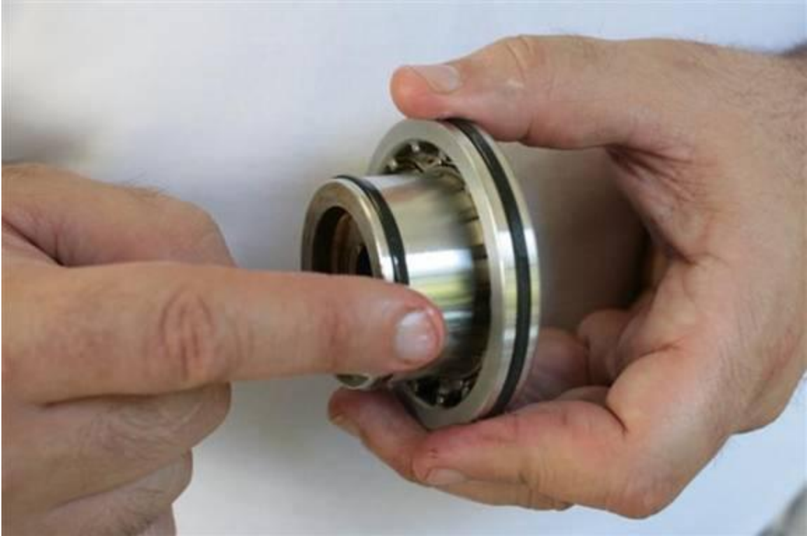
Apply coat of assembly lubricant (engine oil) to vanos piston small Teflon seal and adjacent piston surfaces.
