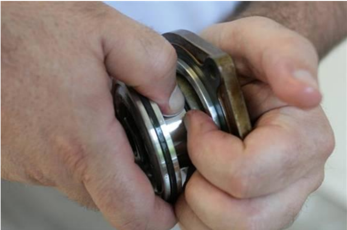
Insert piston small end into cover cylinder inboard side. Insert piston with a
