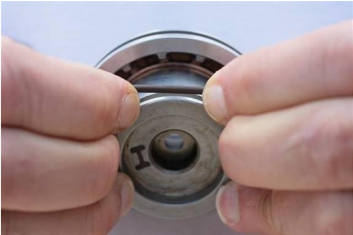
Install small and large O-rings (circular brown) in corresponding piston grooves.
